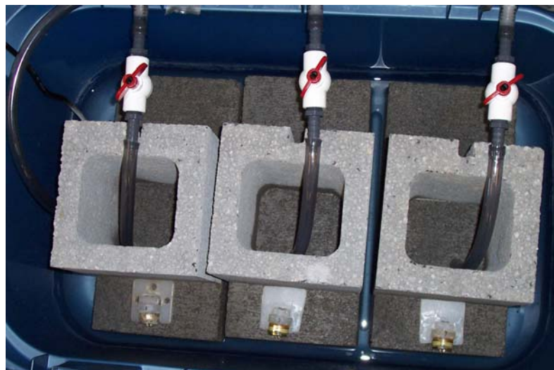
Figure 6. Photograph showing view of artificial springs and electrical resistance sensors in a laboratory setting. Electrical resistance sensors are located at the base of the cinder blocks. Water flows out of the base of the cinder block reservoirs through a narrow crack past the sensors.
