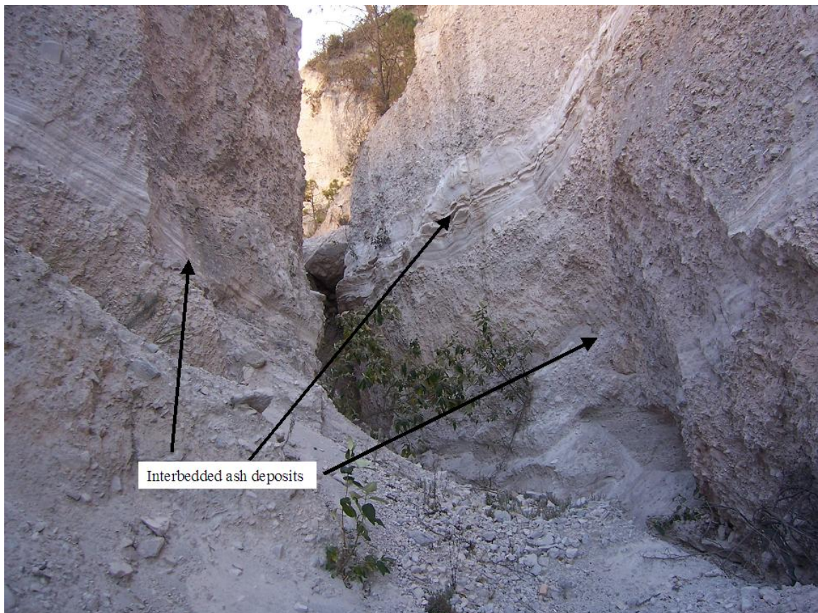
Figure 4.3. Bpi with interbedded ash deposits originating from the north ring. Ash interbeds are 35-50 cm thick at this location.
