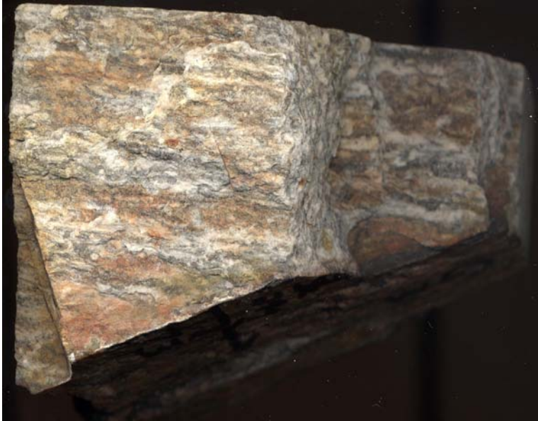
Figure 22. Photograph of hand sample showing lineations on foliation plane. Lineations are defined by light and dark streaks consisting of concentrations of quartz, feldspar, and biotite. This is a sample of orthogneiss. Similar lineations are preserved in other units. Sample measures 10 cm from left to right.
