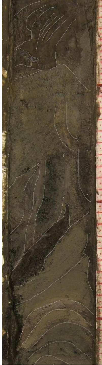
Figure 13. Example of disturbed sediment from core MG07-11. The contorted and broken bedding contacts indicate zones of disturbed sediment. The stratigraphy in this image is most disturbed in the top and middle sections, decreasing to mostly pronounced bowing of the sediment, from coring, near the base (white lines). Red lines are 1 cm apart.
