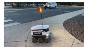
Figure 3: Example of a sidewalk autonomous delivery robot
