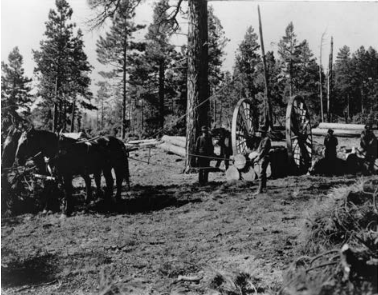
Figure 2.9. Five lumberjacks with a two-draft horse team pulling a Big Wheel cart loaded with logs, circa 1904 to 1910. From Williams Historic Photo Archive, Williams, AZ.
