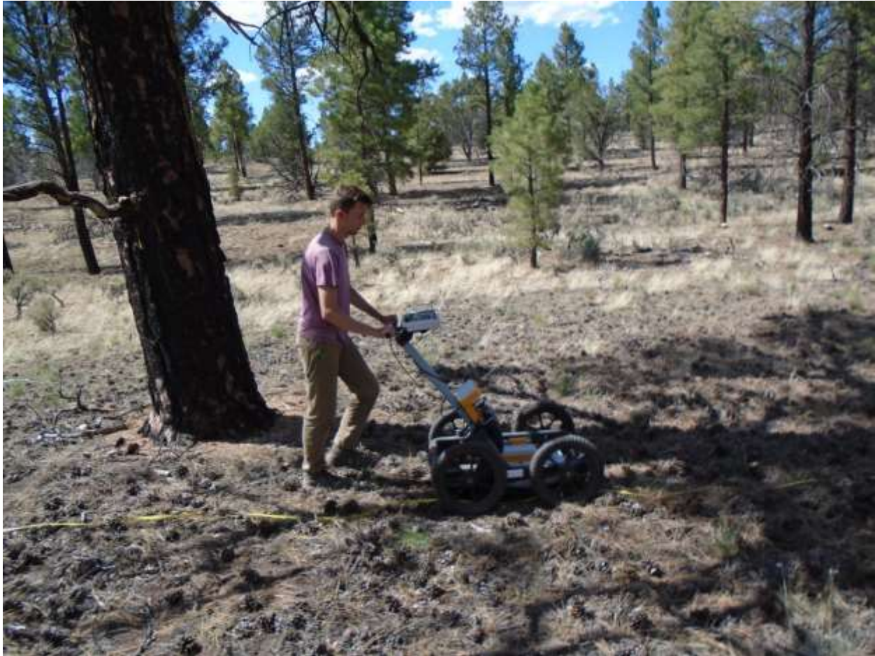
Figure 2: Logan Hick pushing the Ground Penetrating Radar at Locus I. Photo by Nathan Crennan.
